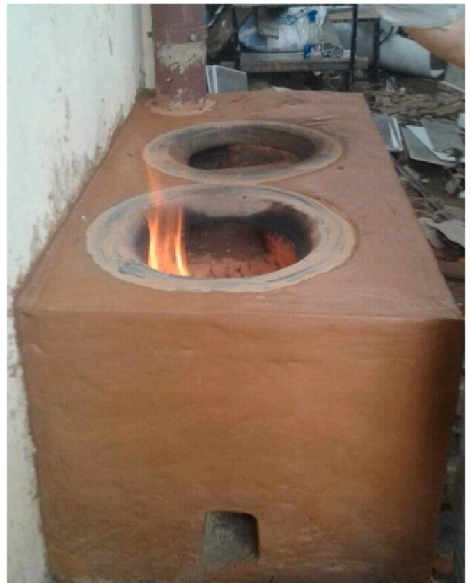
Fig. 4. Improved cooking stove constructed with mud. Source: Author.
