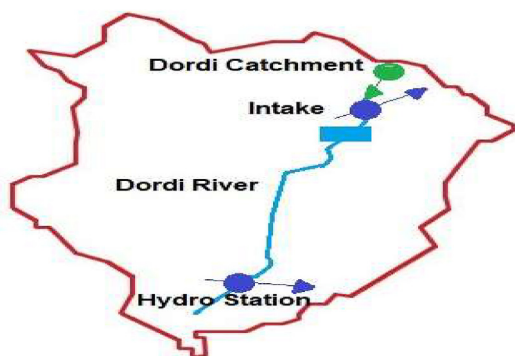
Figure 7. WEAP model set up for the Dordi River.
